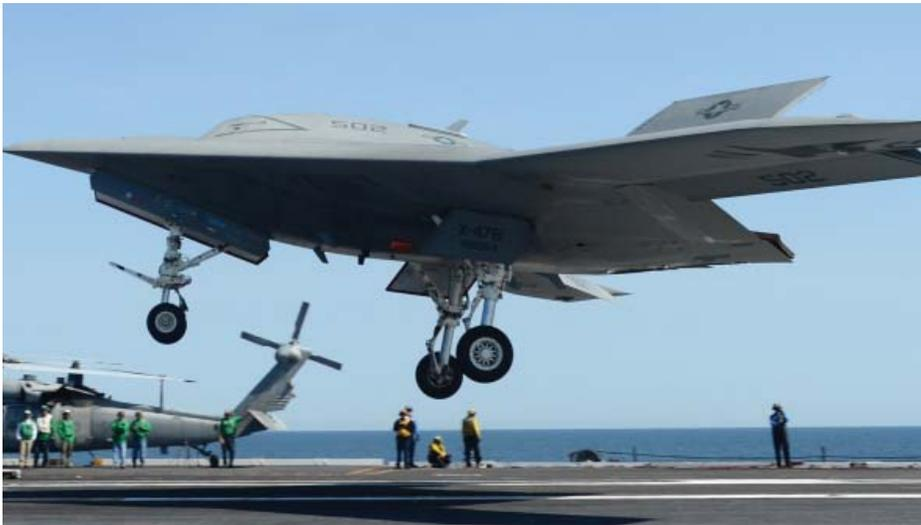
The X-47B unmanned combat air vehicle (UCAV) is a demonstrator stealth carrier-born strike bomber. Similar in concept to the cancelled A-12 Avenger II, the X-47B first flew in 2011, and made its first catapult launch at sea from the USS George H.W. Bush in May 2013. In July 2013, the X-47B completed the first arrested landing
