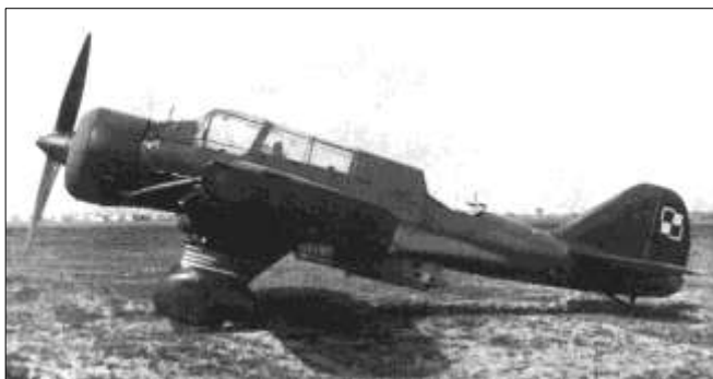
PZL 23A - Along with the earlier version of the Pegasus engine, the "A" had a leading edge slat that was deleted from the "B"
