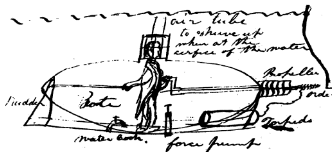
The drawing of the Silas Plowden Halsey boat shows the operator with one hand on a tiller, the other on a crank to turn the propeller and drill bit. A technical "Turtle" clone: there is a "water cock" and a "force pump" at the bottom of the boat and an "air tube to shove up when at the surface of the water." A "torpedo" is attached by a line to the drill.
