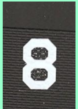
Close Up of the decals on the matte side of the panel showing "silvering"
