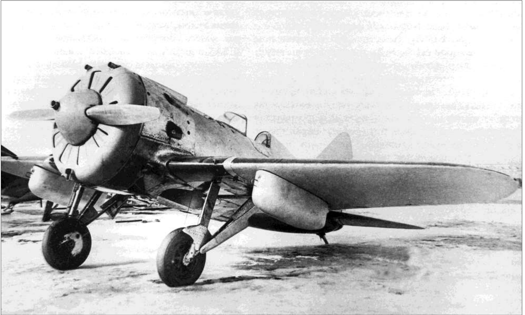
Polikarpov I-16 Type 20, 1021681; a modified I-16 Type 10 equipped with two 200 liter underwing fuel tanks
