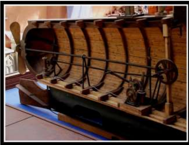
A longitudinal-section of Fulton's 1806 proposed design
