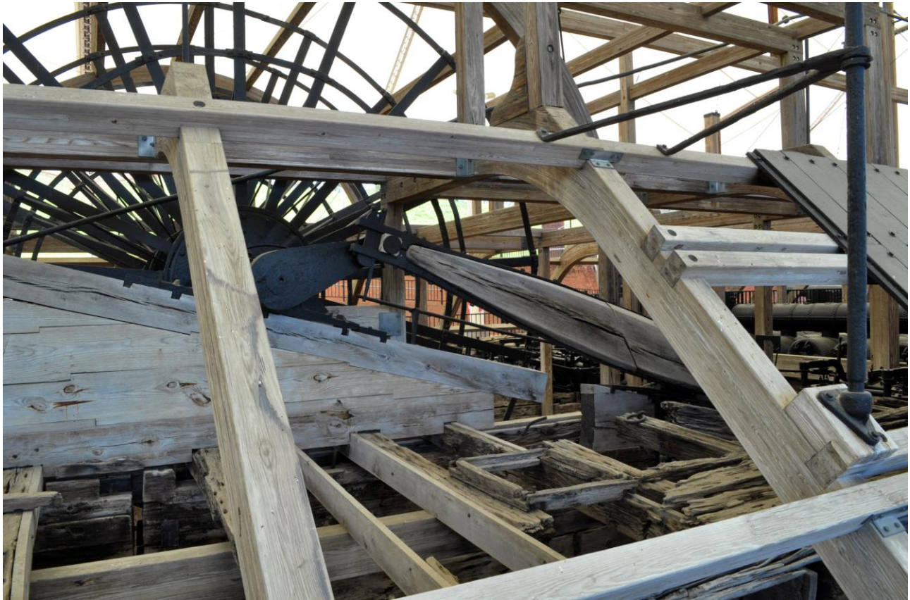
This view highlights the construction of the massive connecting rods.
