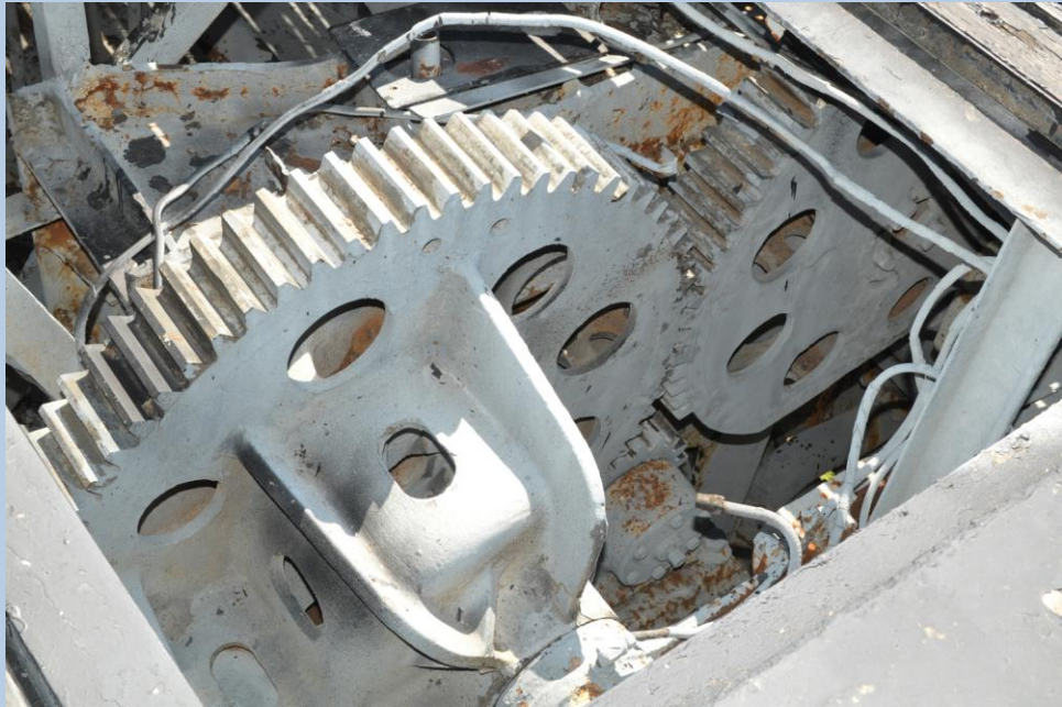
This is the drive gear for the bow planes.
