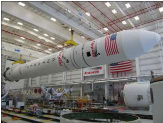
The Antares rocket for Orbital Science's A-ONE inaugural mission is hoisted inside Wallops' Horizontal Integration Facility for placement on its transporter. It will be moved to the launch pad on the morning of Saturday, April 6, 2013.
