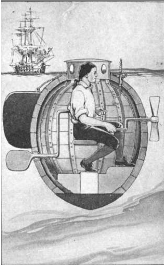
Drawing of a cutaway view of Turtle's interior.
