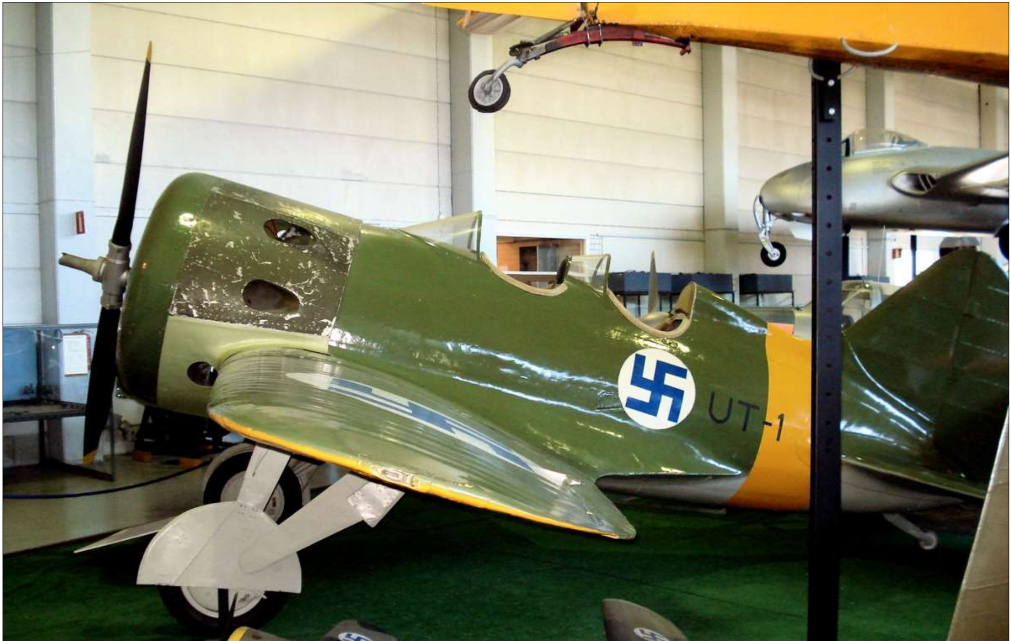
Two-seat I-16 UTI trainer version, with Finnish markings on display in the Finnish Aviation Museum in Vantaa, Finland
