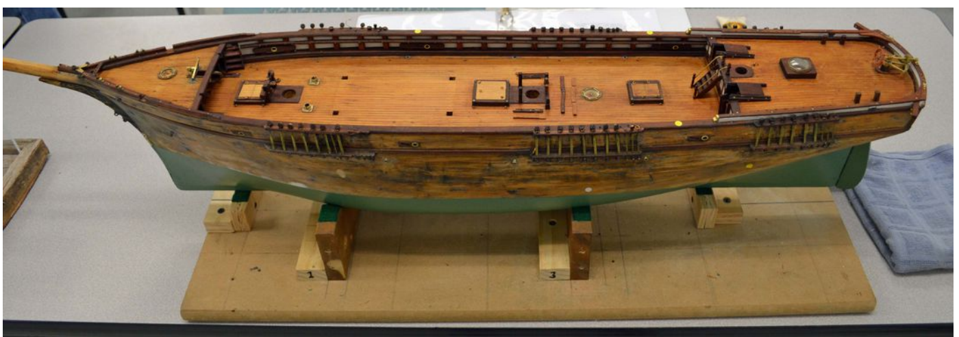
The painting of the hull below the water line has been completed. Above the water line, I will be using Jo Sonja's Artist's Carbon Black Acrylic Gouache (velvet matte finish) and brushing it on. In the picture above, you can see a "test" run that worked out very well. I also masked the waterline using Scotch Brand #811 Removeable Magic Tape. It worked flawlessly.
