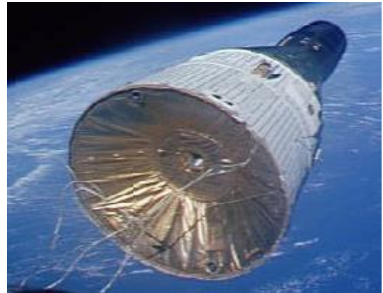
Figure 10: The gold mylar shield at the rear of the Equipment Modules
