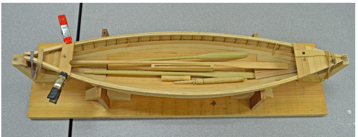
Jack has been studying how these boats maneuver in the hunt on the open sea. As you can see, the planking is coming along nicely. Note the loggerhead and steering oar. Jack is using Erik Ronnberg, Jr's "To Build a Whaleboat, Historical Notes and a Modelmaker's Guide" to assist him in his build.
