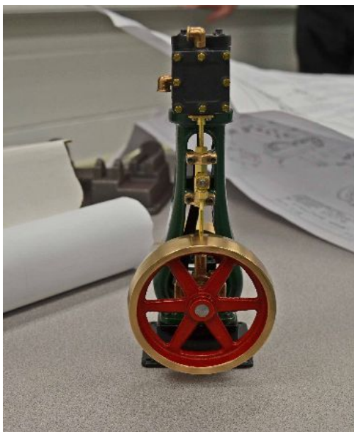
Dave bought Pete Demarest's milling machine and lathe and has gone all out to master it. This is his first effort, a single cylinder vertical engine from a kit. The scale is 1:8 and it runs on compressed air.
