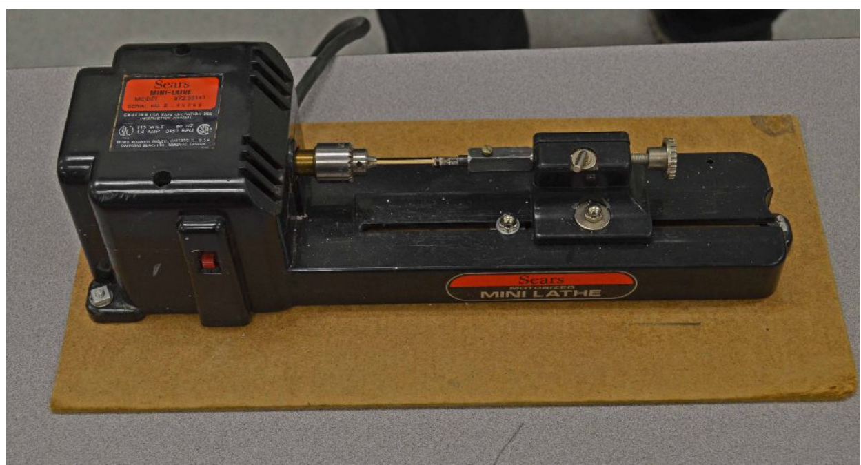
He has adapted a mini lathe into a home made duplicator using brass tubing.
