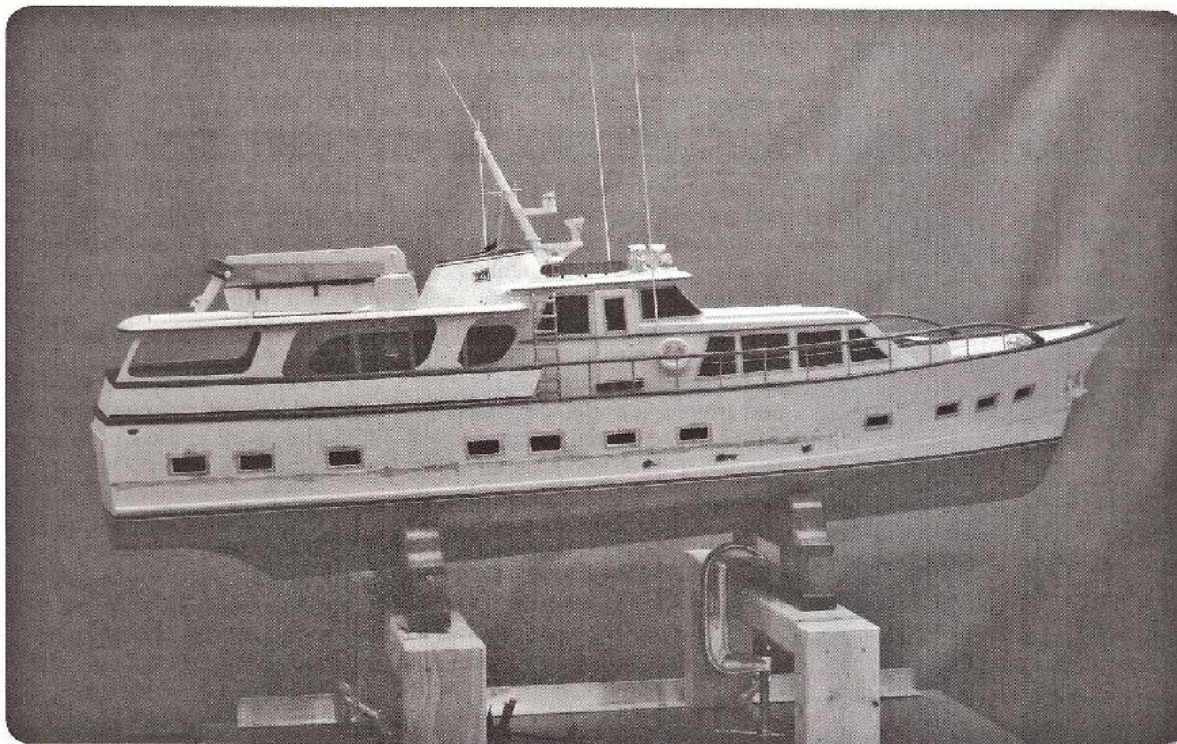
Photo 2. As received, more or less. Port frames, rub rail, props, prop struts, and prop shafts have been removed. Note the bow-high attitude set up by the cradles.
