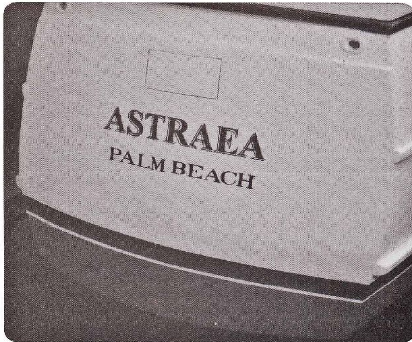
Photo 3. Transom lettering. Hail port done with dry transfers. Name is a custom decal made from computer-generated artwork for the basic letters. Shadowing was added to the artwork with a fine pen before printing completed image on decal paper.
