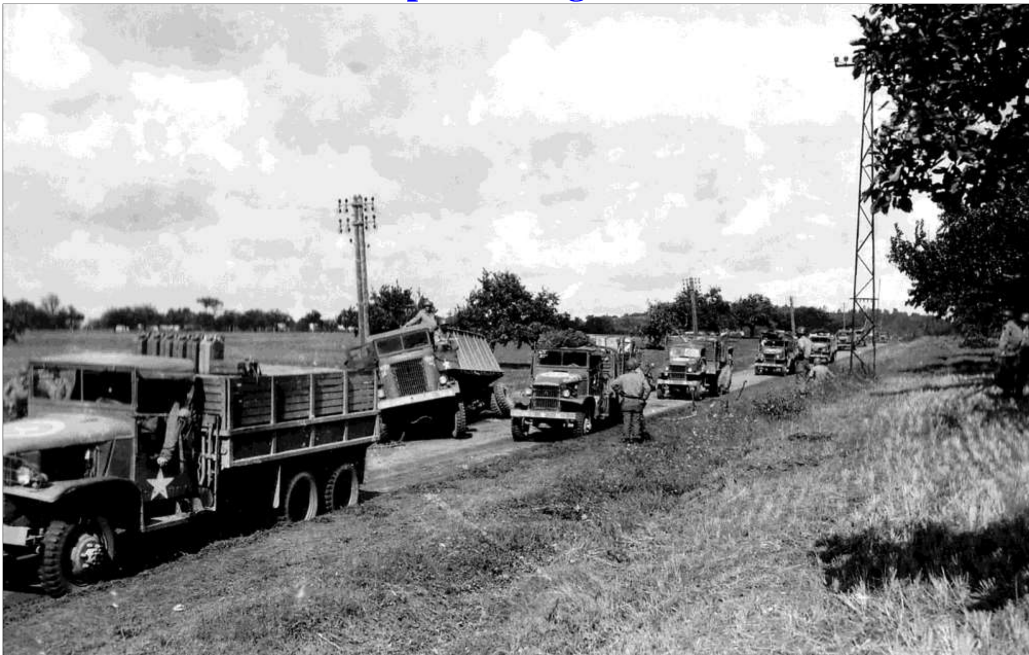
A truck of the US Army 'Red Ball Express' fell into a ditch at the side of a road; GMC CCKW 2 1/2-ton 6x6 transports lined the road as a GMC AFKWX tractor struggled to free itself, France, 1944
