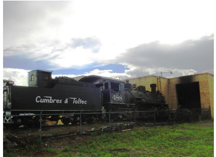
Engine 488 out back of its storage shed with the fire just burning enough to keep the boiler heated overnight.
