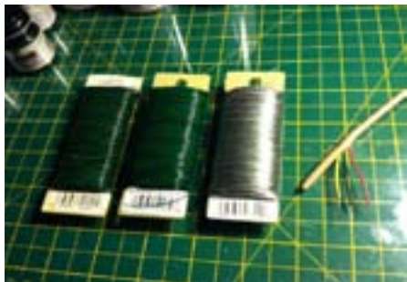
Several gauges of wire were used to detail the engine compartment. Mike Turco photo.
